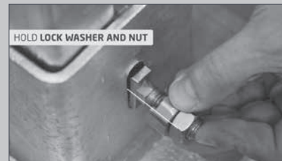
Insert T-lock through component and profile, position as required.
