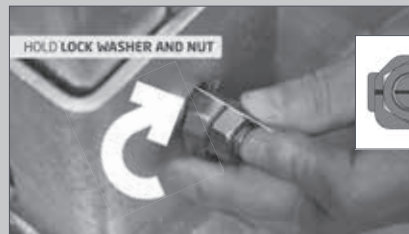
Turn T-lock 90° (marking notch stands diagonally to the elongated hole).
