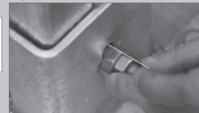
Tilt forward T-lock, so that guide wedge of Lock washer snaps in elongated hole. Then tighten by screwing the nut (hand-tight).
